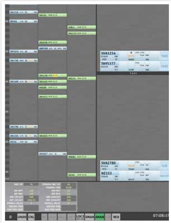
OPTAMOS is highly flexible. Runway changes, closures, including temporary closure of taxiways, can easily be taken into consideration in order to deliver precise TSATs. OPTAMOS can handle remote deicing situations and remote parking, as well as flow management restrictions from regulating bodies.
