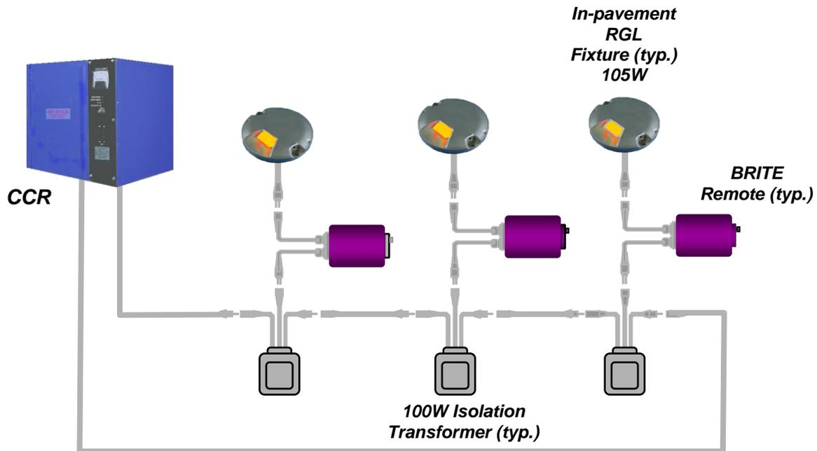
**Figure 1: Un-monitored in-pavement RGL system.**
