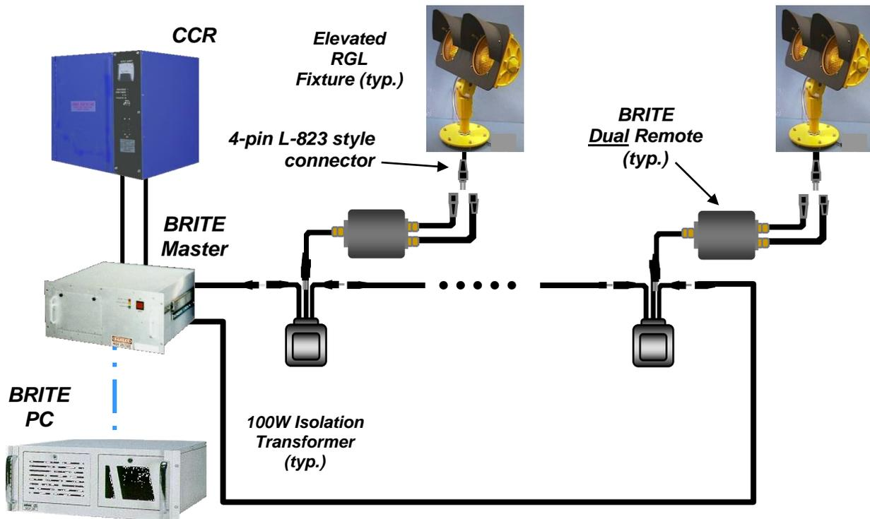
**Figure 4: Monitored Elevated RGL system.**
