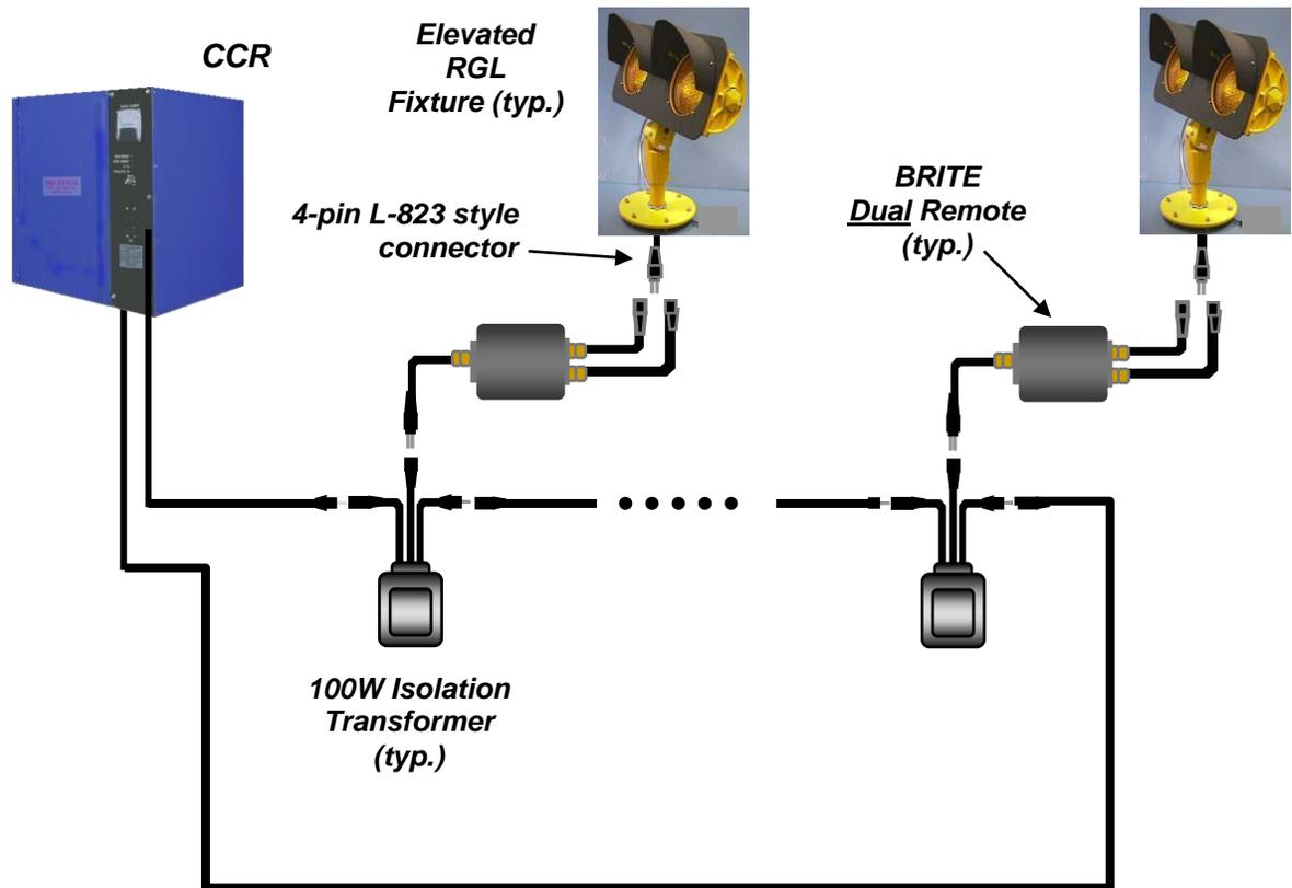
Figure 2: Un-monitored elevated RGL system.
