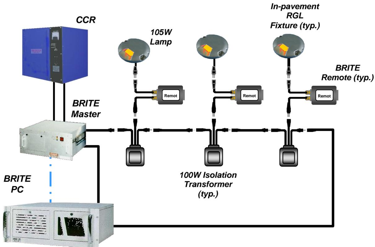
Figure 3: Monitored in-pavement RGL system.
