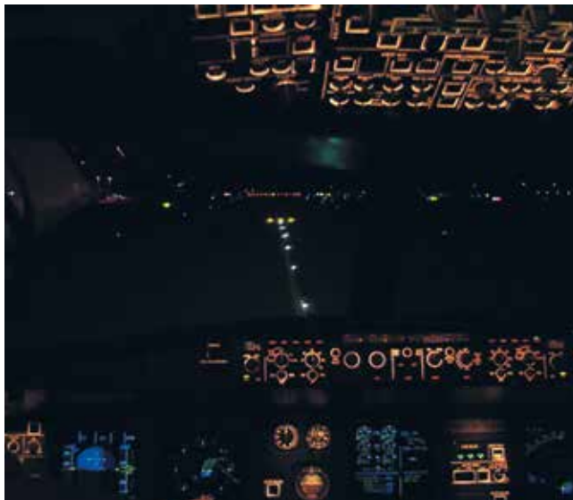
Cockpit view: visual guidance with AGLAS individual lamp control.
