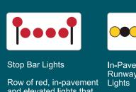
and elevated lights that, when illuminated, designate a runway hold flashing yellow position. NEVER lights at runway CROSS AN holding positions holding positions indicating an active ILLUMINATED RED
