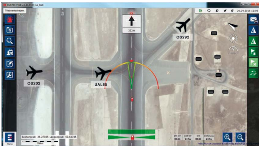
▲ Figure 18 – Airport Vehicle Onboard Navigation System (Source: www.rosenbauer.com )
