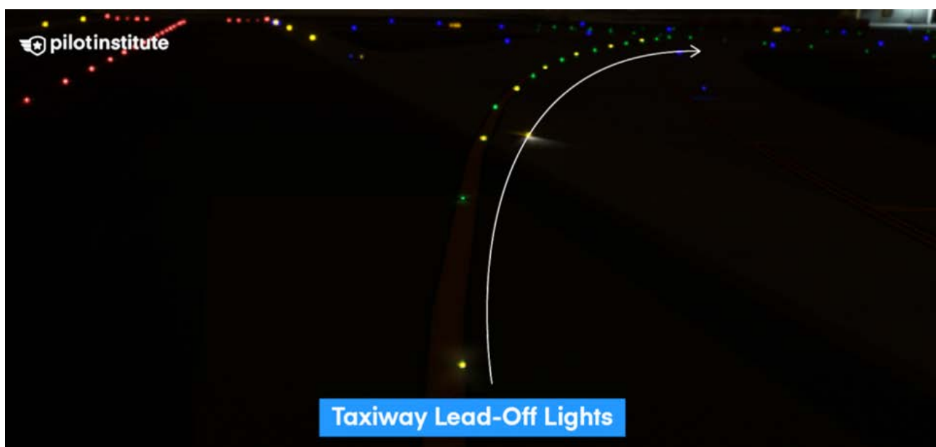
▲ Figure 16 – Taxiway Lead-off Centerline lights (Source: pilotinstitute.com)
