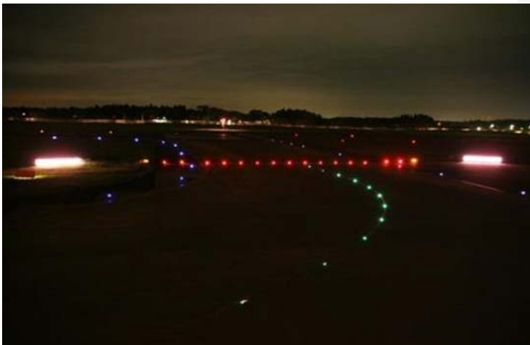
◀ Figure 14 – Stop bar lights are an effective barrier, but often used only in LVC (Source: ICAO)
