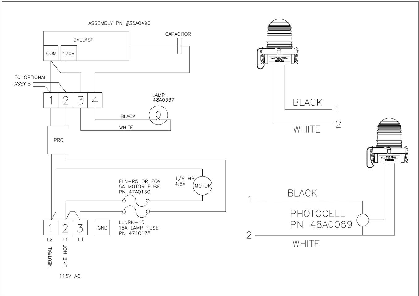
Figure 14. Internal Wiring Schematic
