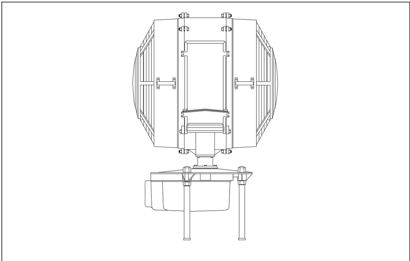
Figure 1. L-802A Rotating Beacon
