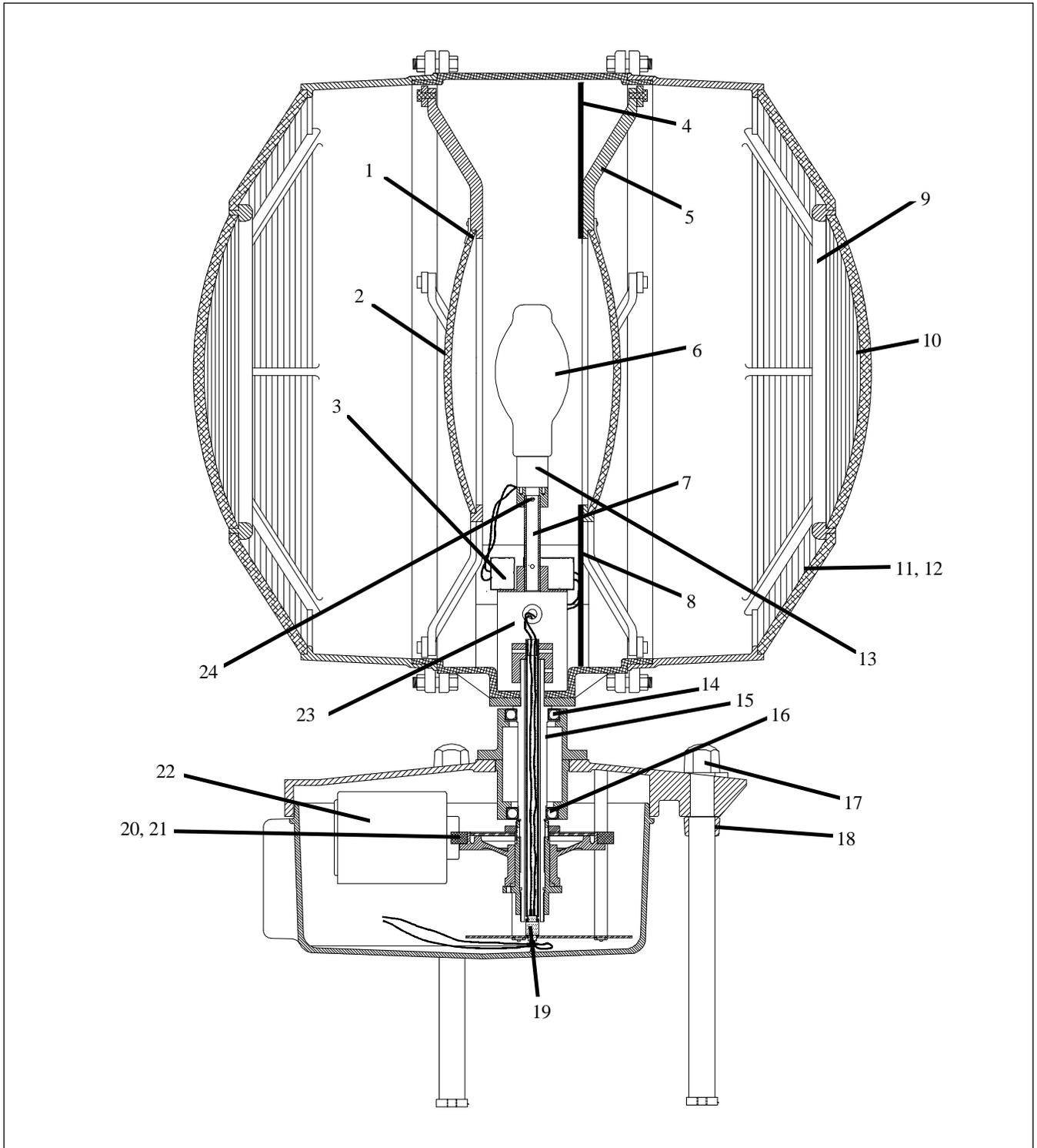
Figure 13. L-802A 36-Inch Rotating Beacon (Part 1 of 2)
