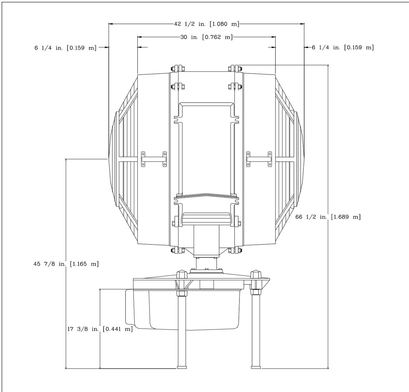
Figure 3. Overall Mounting Dimensions
