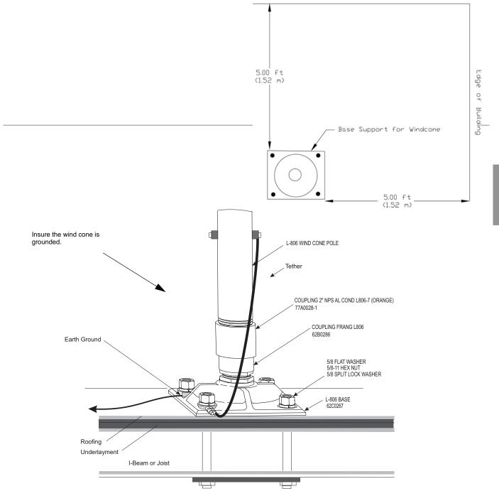
The base support is designed to use 5/8-inch (15.87 mm)-diameter bolts. The mounting hardware is supplied by the contractor. See Figure 11 and Table 3.
