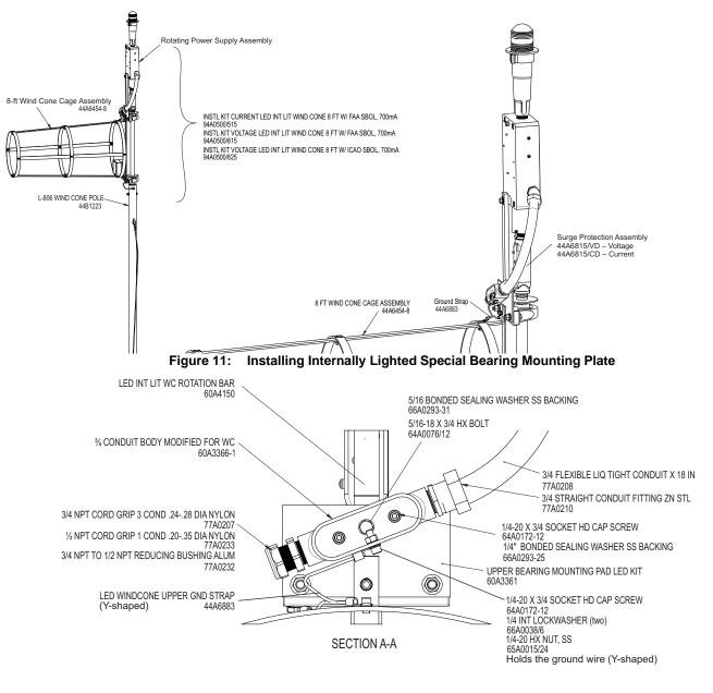
2. Mount the special Bearing Mounting Plate (See Figure 11) supplied with the Internal Light Kit along with the L-Shape Cage Strap, to the top of the throat ring.
