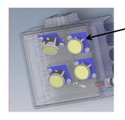
The 1000mA Light Engine 44A6786 uses a star shaped PCB over a square mounting plate.
