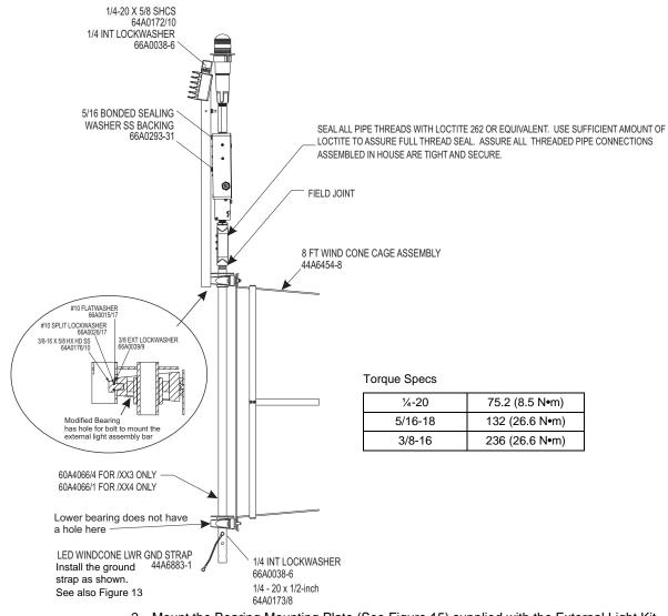
Figure 15: Installing Externally Lighted Assembly Details
