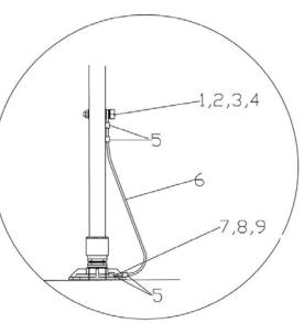
When mounting the L-806 wind cone on a roof, a tether must be installed. See Figure 20. Refer to Table 3 for tether installation parts. To install a tether (contractor-supplied), perform the following procedure:
