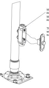
WIND CONE POLE SWITCH ASSEMBLY VOLTAGE DRIVEN 44A7339-20 WIND CONE POLE SWITCH ASSEMBLY CURRENT 44A7339-10
