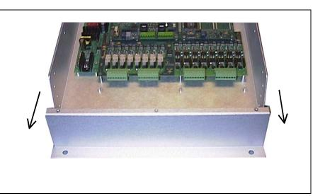
Figure 6: Removal of bottom access plate
